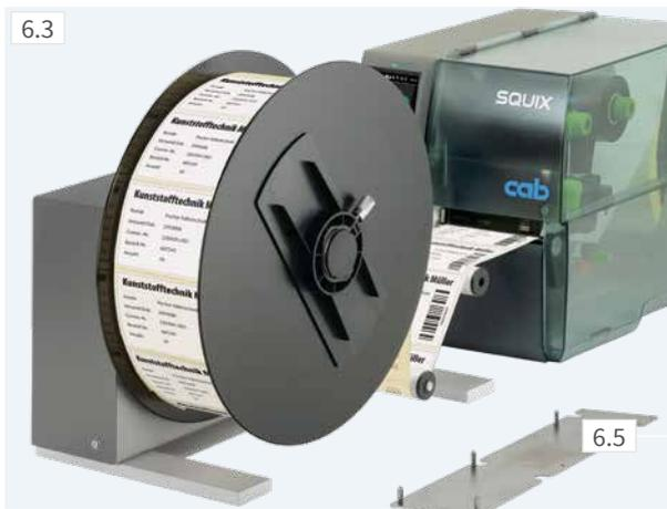
**External ER4, ER6 rewinders**, power supply built in. Label webs wound outside or inside are wound consistently and tight by electronic control, with the help of a pendulum arm. They operate also with printers other than cab.
