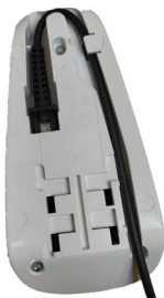
Figure 5 - Options for routing the DC cord
