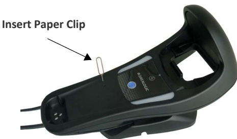
Figure 8 - Disconnecting the Cable
