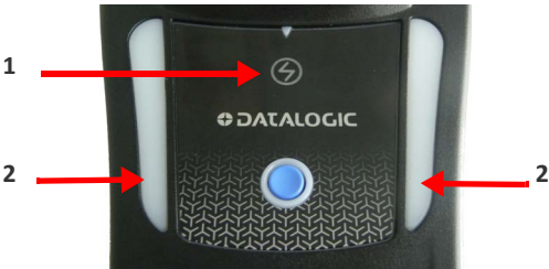
Figure 12 - Gryphon Base LEDs
