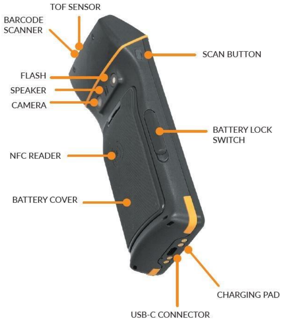
Picture 7 Features of Nordic ID HH83 (back side)
